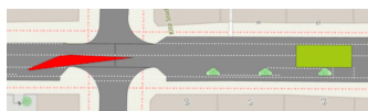
Fig. 10: Comparison of roadwork measured by the system (red) and Geoport Berlin [18] entry (green), registered half a block away from the actual position, therefore failing to show the intersection blockage
