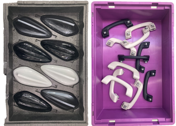
Fig. 1. Automotive antenna covers (left) and interior handles (right) in storage containers, that enforce structured and unstructured positions.
