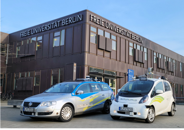
Fig. 6. Autonomous vehicles used to test the proposed method. Both vehicles are equipped with 360° LiDAR, Applanix POS LV position and orientation system, and V2X communication devices.
