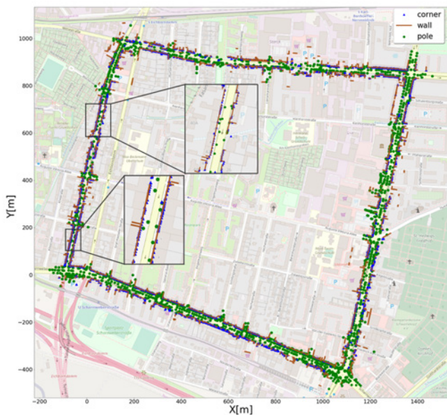
Fig. 5. "SAFARI" test field for automated and connected driving in Berlin, the main road is about 5.6 km. The zoomed in view shows the area where only a few poles exist but plenty of corners and walls can be detected.
